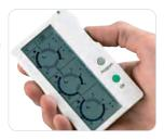
The MB programmer communicates with the heaters and controls a comfort or setback thermostat as per the times set in the programmer.
